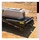
The available mega ramps provide a loading surface that covers almost the complete deck width, to provide maximium stability and loading options flexibility.
