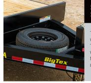
The 140A comes standard with an inegrated Storage Tray in the tongue area as well as a Spare Tire Mount for convenient storage during transit.
